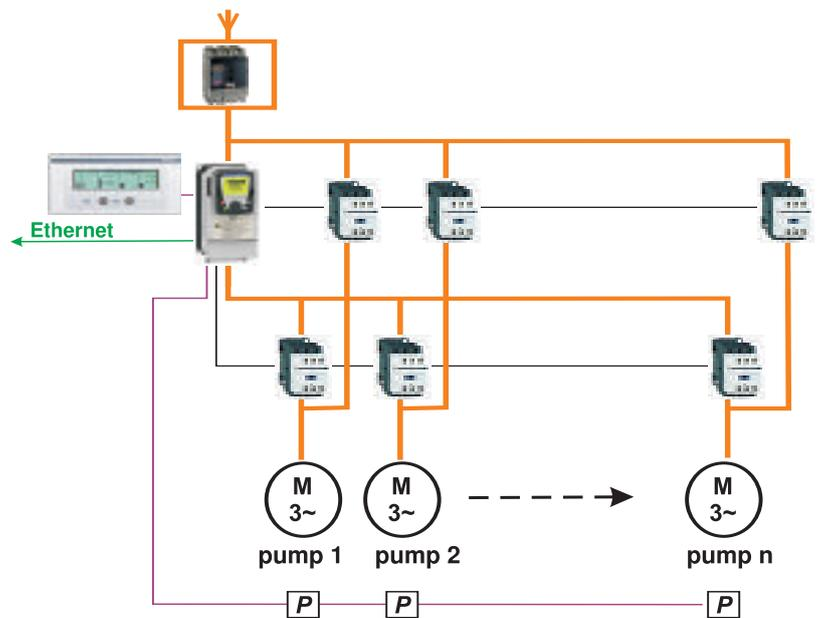
↑ Fig. 34 Solution 2 from a speed drive
