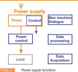
As illustrated in the diagram ( $\Rightarrow$  *Fig. 2*), an electrical power supply is divided into two units.
