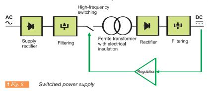
A loop feedback controls the high-frequency switch cycle time to ensure the requisite regulation characteristic ( $\Rightarrow$  *Fig.* 9).
